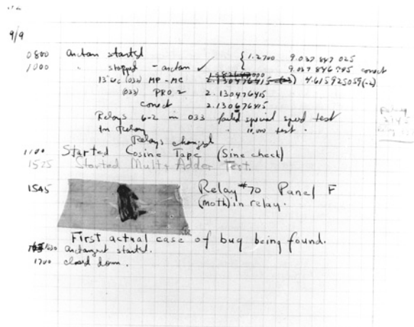
FIGURE C.3 A real hardware bug! [Courtesy of the Naval Surface Warfare Center, Dahlgren, VA., 1988. – U.S. Naval Historical Center Online Library Photograph.]
